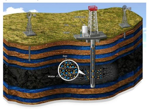
Figure 23: Coal seam gas and its extraction <sup>326</sup>
